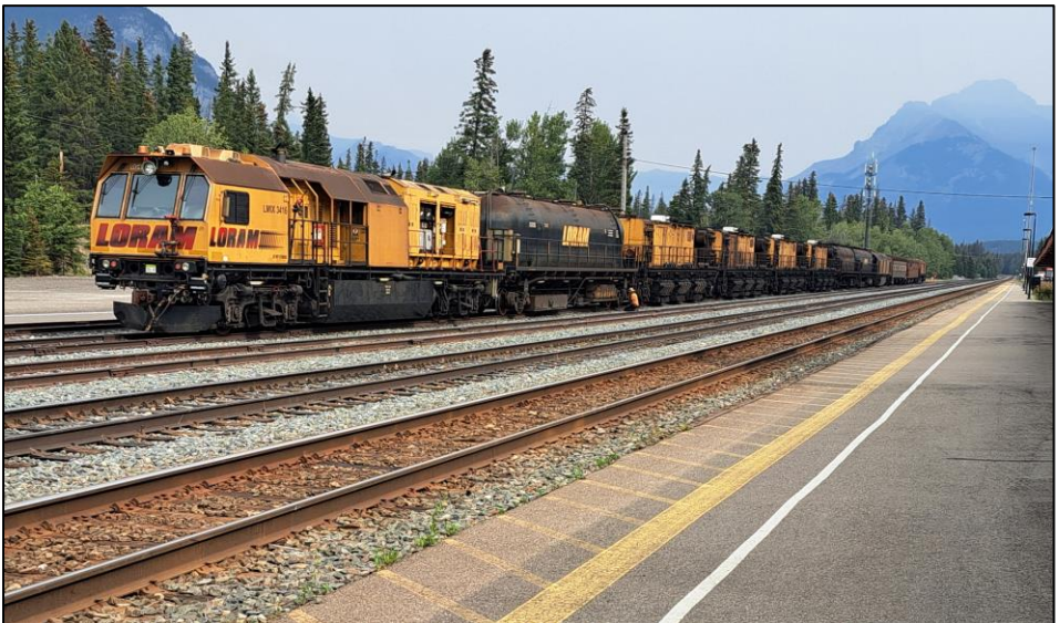
Loram Rail head grinding and reprofiling train stabled in the sidings at Banff
